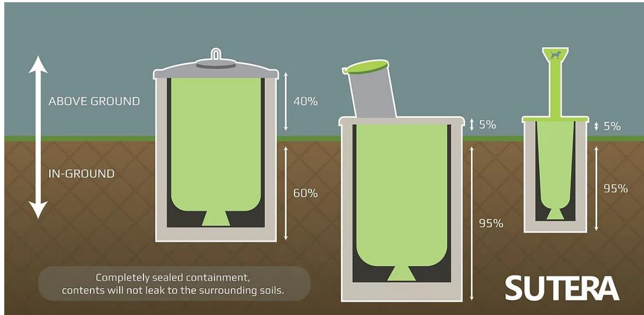
Figure 34: Profile of SUTERA In-Ground Containers
