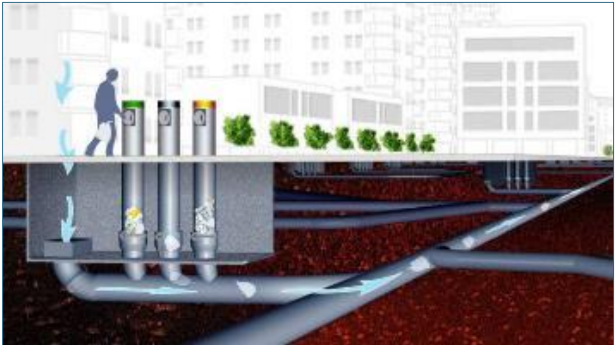
Figure 30: Bossnett Underground Waste System
