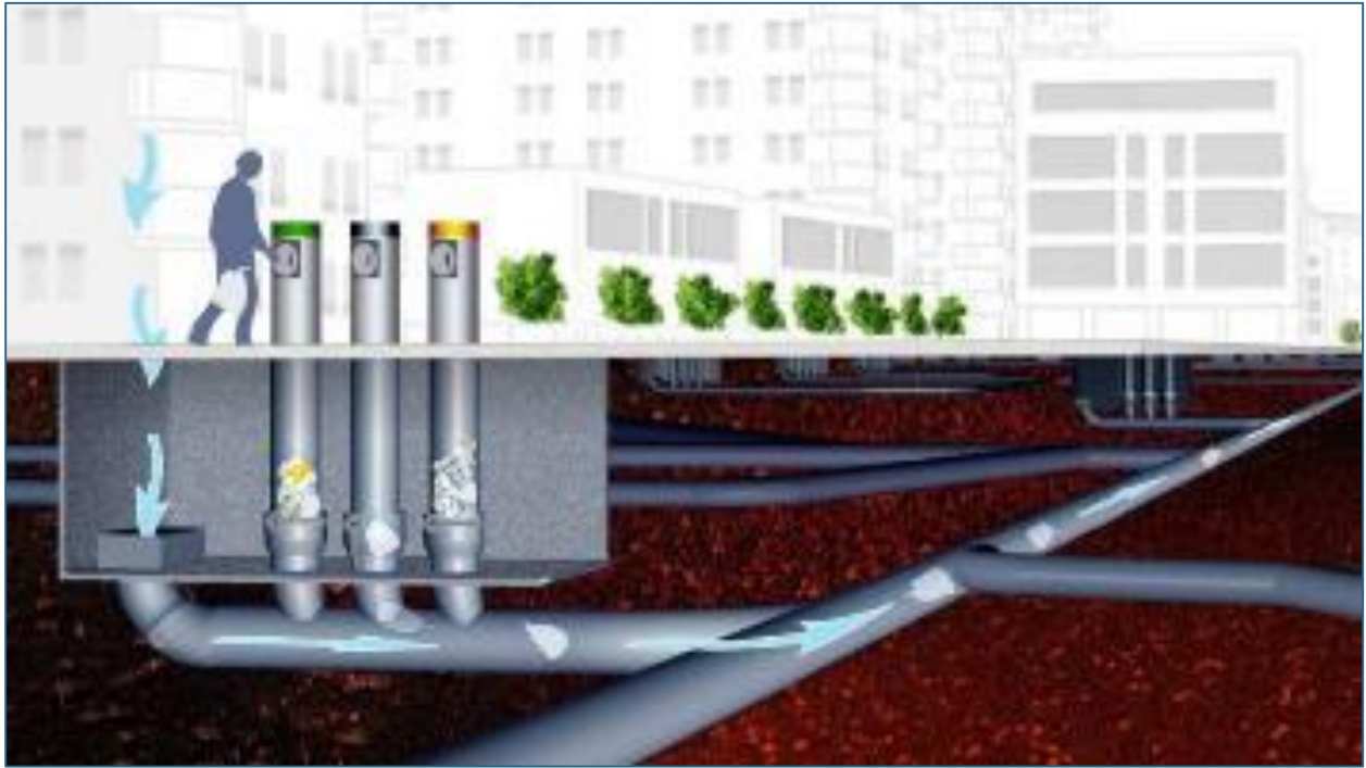
Figure 30: Bossnett Underground Waste System
