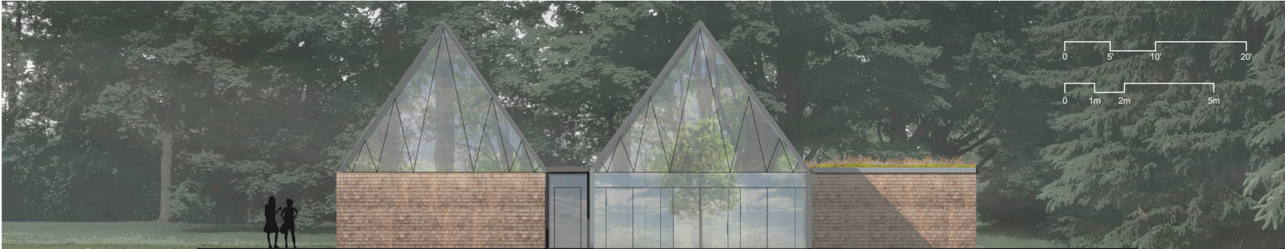
Conservatory east elevation with wood shingles and glass
