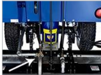
Advanced Water System — AWS™ Regulates amount of water dispensed onto the ice relative to machine speed for efficient and even application. *optional equipment
