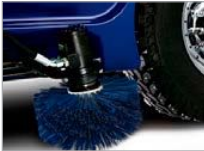
Zamboni Power Brush™ Wider brush path reaches higher on the dasher board kick plate for superior cleaning power. *optional equipment
