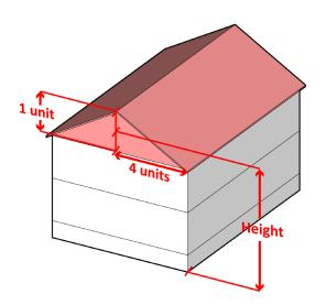
Figure 27. Illustrative Diagram for Pitched Roof
