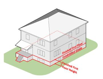
**Figure 29.** Illustrative Diagram for Height, Finished First Floor
