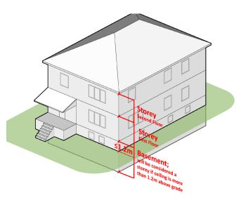
Figure 30. Illustrative Diagram for Storey
