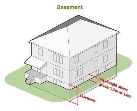
Figure 25. Illustrative Diagram for Basement
