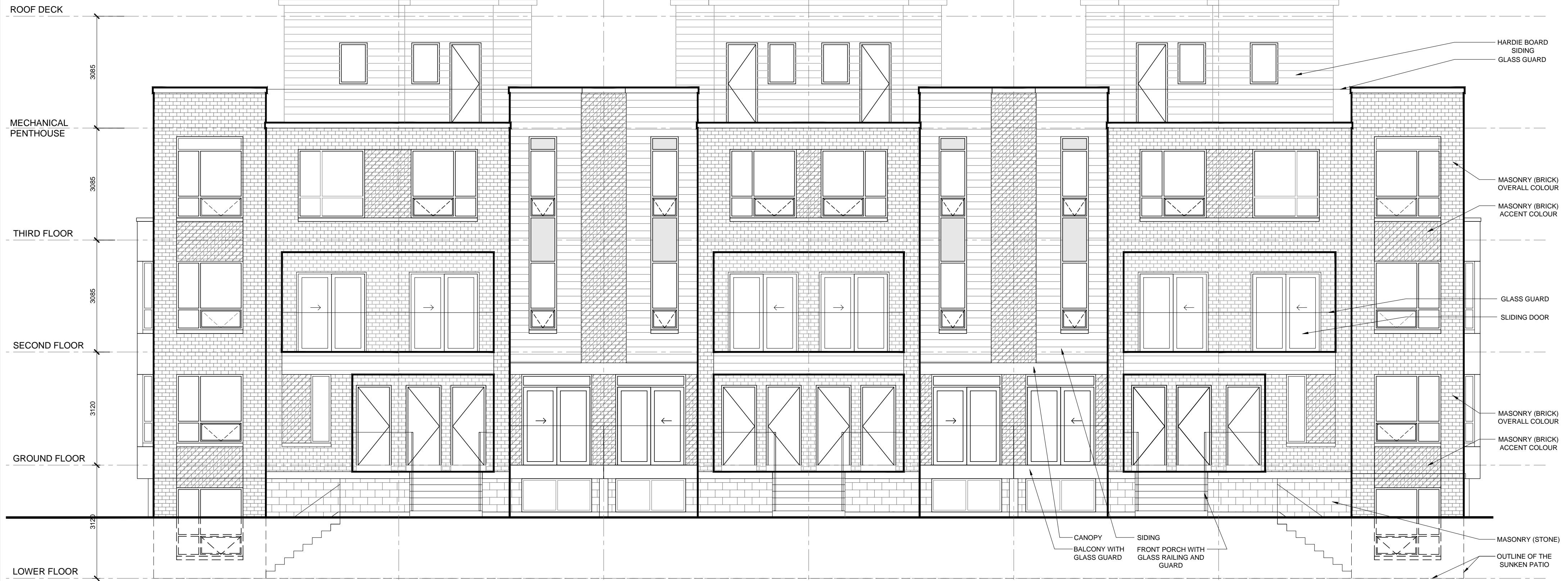
1 FRONT ELEVATION - BLOCKS 3, 4, 6, 11 AND 12 A400 SCALE: 1:75
