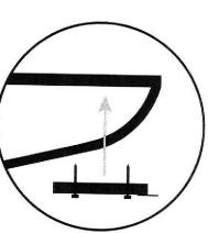
1" X 1" tubing brackets to be bolted to the wall every six feet along the top of the awning using 3/8" X 4" lag bolts and washers. Additional brackets will be used to secure the bottom of the awning
