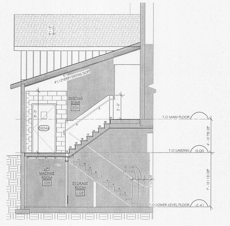
4 EXISTING STAIR SECTION A200 SCALE: 1/4" = 1'-0"
