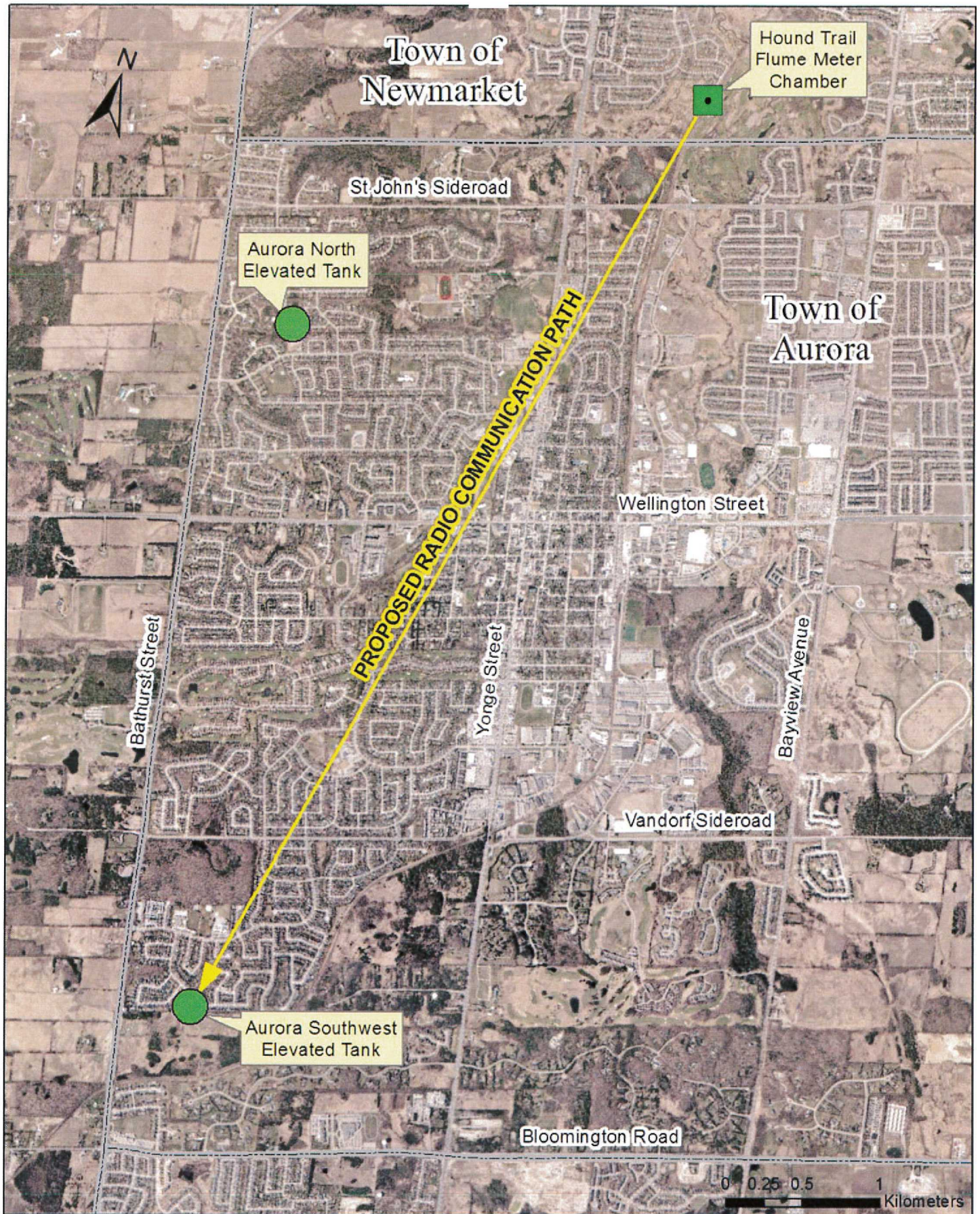
Radio Communication Path From Hound Trail Flume Meter Chamber to Aurora Southwest Elevated Tank
